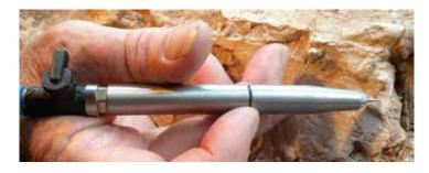
HW-1 - Needle holder and needle - Hard metal (2mm) or steel (1.3 mm) diameter
