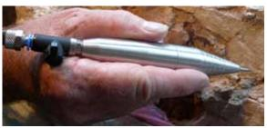
HW-70 The most versitile flying piston pneumatic air scribe because there are 3 different diameter heads and needles offered making it good for a wide range of work. It has a well balanced great feel. Hose, connectors and in line regulator included. Supplied with choice of 1.3 mm, 2 mm or 3 mm diameter standard length tip
