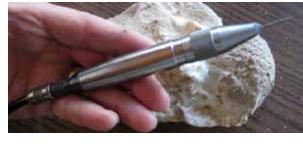
HW-322 For ultra-fine work usually under a microscope runs at 5 psi up to max 26 psi so in line regulator is required to keep pressure very low. Supplied with hose, connectors, in line regulator and two springs, hard and soft that provide versatility in the action of the tool. Standard sticks out 7 mm. Tool - choice of 1.3 mm head/tip or 2mm head/tip Tool with both size heads/tips
